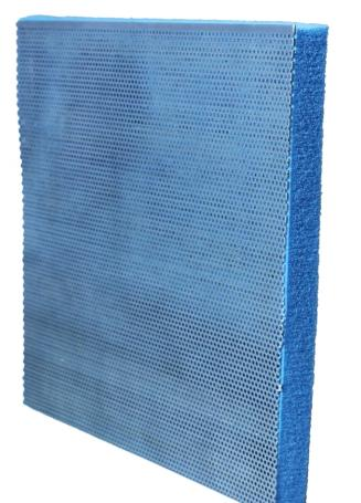
The combination of the elements that make up the **Metapanel Insulation Low Frequency** product makes it possible to have a resonant mechanism, which makes the soundproofing power particularly efficient in very specific frequencies, from 500 to 2000 Hz. The resonant phenomenon can be appropriately designed and adjusted to intervene in the most interesting frequency ranges depending on the application.
