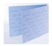
KWO® CellFlon® Sheet Blue structured sheets with PTFE microspheres and hollow glass. For applications with limited bolt load or uneven flange. For sealing chemicals with pH (0-14).
